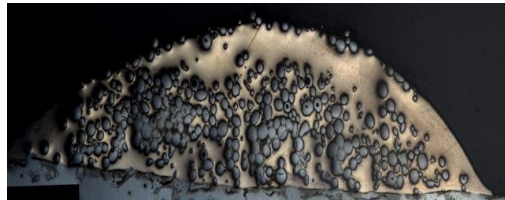
Copper on steel with WC ceramic added
